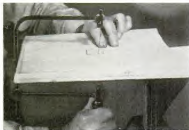
OPENING can be cut in the center of a large piece of work by first drilling pilot holes at four corners
